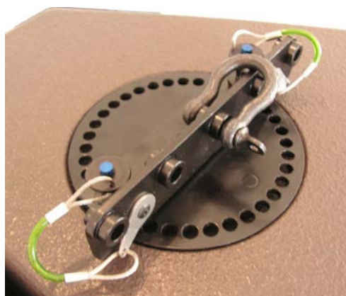
(4) Two locking pins are used to secure the XTLIFTBAR. Shackle locations (front to back) provide +18, +11, +3, -5, -13 degree tilt angles, respectively
