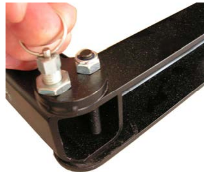
(4) Release pivoting arm locking pin
