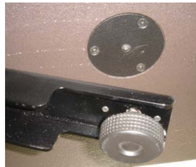
(6) Rotate the pivoting arm into position
