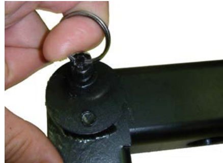
(2) Release pivoting arm locking pin
