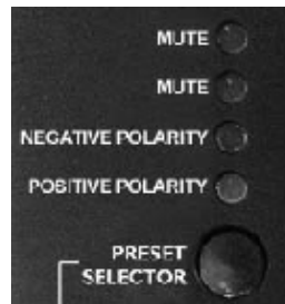
Figure 8: SB15P preset selector switch closeup
